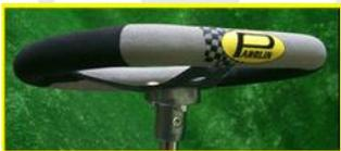
The seat is manufactured in fiberglass and engineered using the latest ergonomic techniques. It also presents a controlled torsion stiffness.
